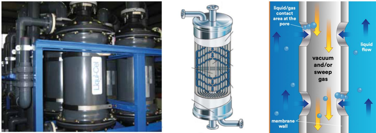
Figure 4. Images of (left) 3M-Liqui-Cel® membrane contactor, (middle) hollow-fiber configuration within contactor, and (right) gas removal process within a single hollow fiber (Images from 3M™).
